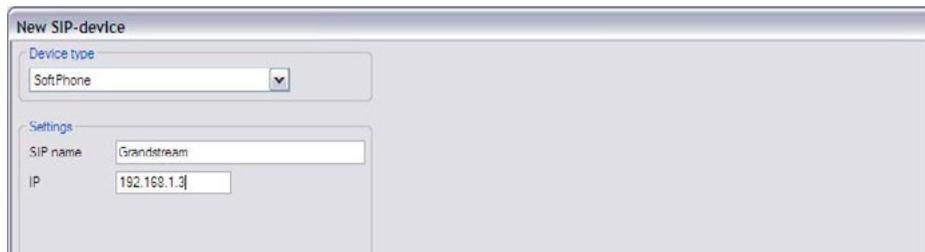
The screenshot shows a dialog box titled "New SIP-device". It has two main sections: "Device type" and "Settings". In the "Device type" section, a dropdown menu is set to "SoftPhone". In the "Settings" section, there are two text input fields: "SIP name" with the value "Grandstream" and "IP" with the value "192.168.1.3".
