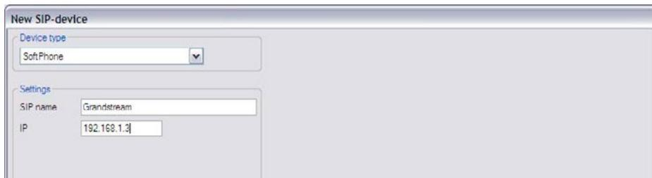
The screenshot shows a dialog box titled "New SIP-device". Under the "Device type" section, a dropdown menu is set to "SoftPhone". Under the "Settings" section, there are two input fields: "SIP name" with the value "Grandstream" and "IP" with the value "192.168.1.3".
