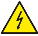
Dangerous voltage: the lightning symbol with an arrow at the end, placed within a triangle, indicates non-insulated, dangerous voltage within the product, which may cause electric shock.
